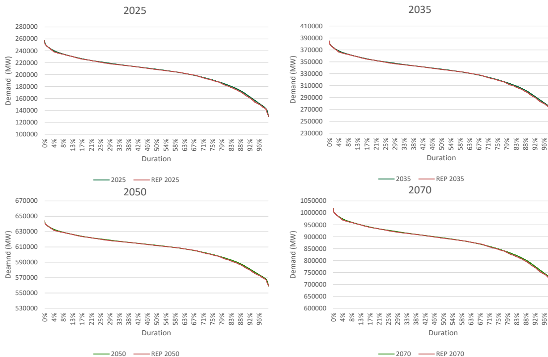
Figure 56: Projected demand load duration curve and the load duration curve for the representative days
